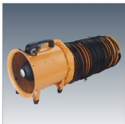
OPTIONAL FLEXIBLE DUCT ● PVC fire retardant with operation temperature 150°C ● extended length to 10m, 15m, by connecting 5m/unit ducts
